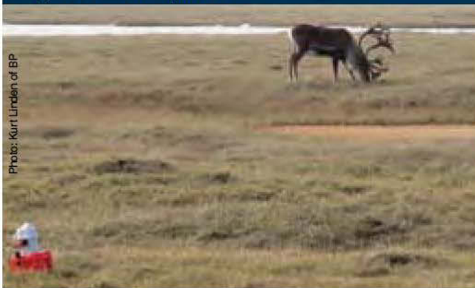
A Sercel UNITE remote acquisition unit with a single analog geophone sitting on its external battery in Alaska.
