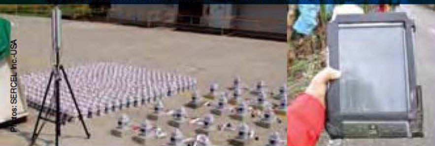
Sercel harvesting antenna and remote acquisition units (RAUs) during the pre-project check and configure process. A hand-held wireless harvester downloads seismic data.
