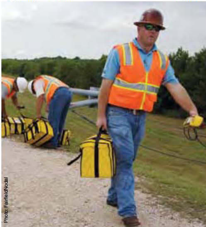
One man can easily carry a FairfieldNodal ZLand node six-pack and the hand-held terminal to start them.
